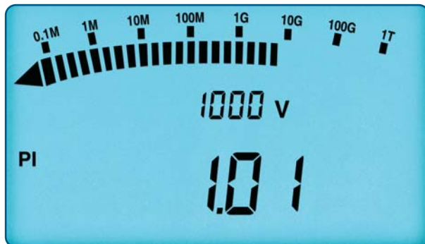
Automatic calculation and display of PI Ratio
