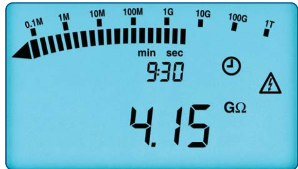
Automatic calculation and display of DAR ratio
