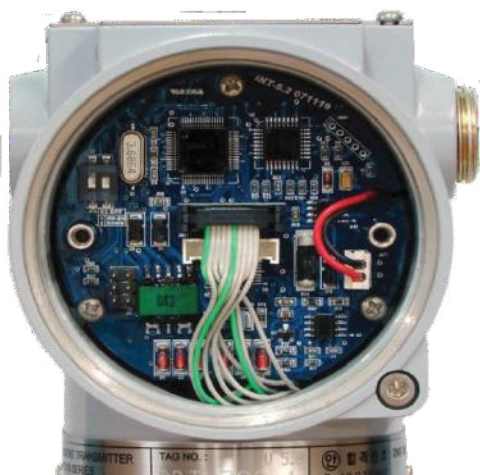
CPU Module Fail Mode, EEPROM-Write Selection Jumper Switch
