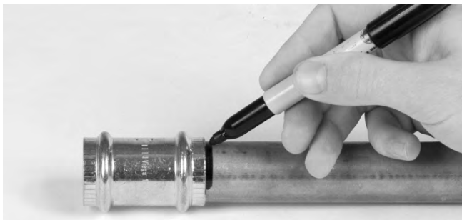
Figure 8 – Marking the Tubing After Fully Inserting Tube
