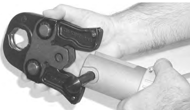
Figure 5 – Pulling The Jaw Set Mounting Pin Out
