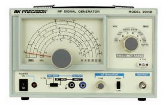
The 2005B supplies sine wave outputs from 100 kHz to 150 MHz (harmonics usable to 450 MHz) at up to 100 mV (RMS). The output can be amplitude modulated with an internal 1 kHz signal or with an external audio signal up to 1 V (RMS). An external crystal can be plugged in for precise frequency control. The output is provided via a BNC female connector.
