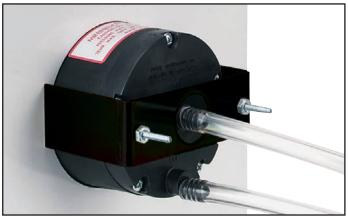
Mounting hardware is supplied with the Minihelic® II gage for panel mounting through a single hole, 2-5/8" (67 mm) in diameter. Panel thickness up to 1/2" (13 mm) can be accommodated with the hardware supplied. If necessary, surface mounting of the gage can be accomplished by means of two 4-40 screws into the tapped mounting bracket stud holes in the rear of the gage. Surface mounting requires clearance holes in the panel for the two pressure taps.
