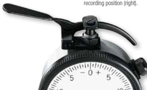
Maximum Hand in at-rest position with indicator hand (left), and in recording position (right).
