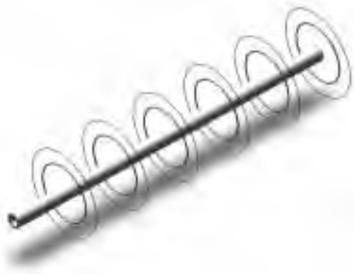
Figure 1 – The field emitted by a charged line.
