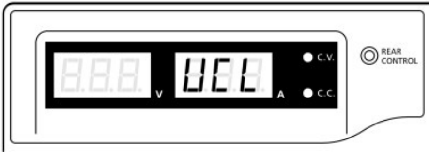
Figure 12 – Upper Current Limit
