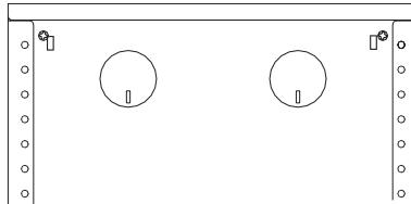
14. Fit the Keyslots in the top corners of the 17A00-9 Assembly onto these screws and tighten.
