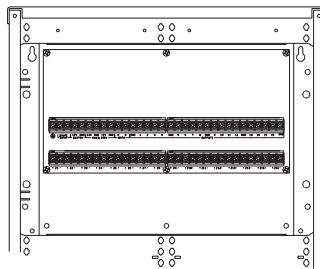
12. Apply the Wiring Diagram Label (17A02-1) onto the inside of the Service Center Enclosure cover and apply the "Leviton Automation Inside" label onto the outside of the cover.
