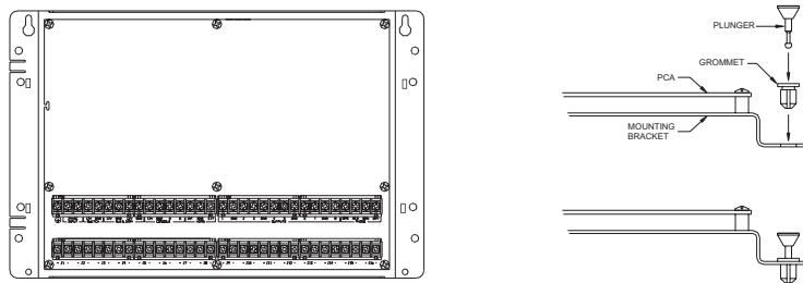
10. Align the assembly with the holes in the back of the Service Center Enclosure and push the grommet into the holes.
