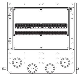
4. Apply the Wiring Diagram Label (17A02-1) onto the inside of the Structured Media Center cover and apply the "Leviton Automation Inside" label onto the outside of the cover.
