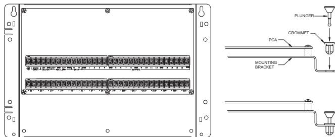
2. Align the assembly with the holes in the back of the Structured Media Center and push the grommet into the holes.
