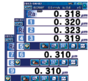
Trace display: the ten latest measurement results using the same parameter
