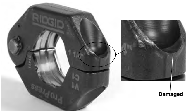
Figure 13 – Damaged Ring Pocket
