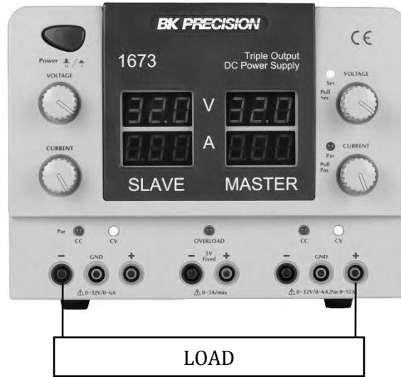
Figure 5 – Series Tracking Mode Load Connection
