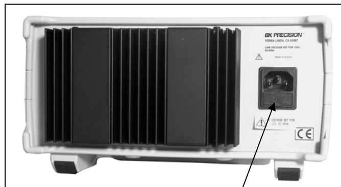
Figure 17. Line voltage conversion switch, determined by fuse holder arrow position.
