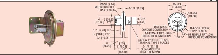
The unique electric switch design in the 1640 is another Dwyer Instruments, Inc. innovation. The Dwyer® Model 1640 Differential Pressure Switch resembles the Series 1630 switches. However, the 1640 is equipped with a single pole, double throw floating contact switch (not snap acting) so it functions as a null switch.
