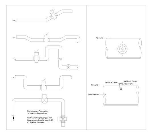
At flowmeter upstream, there should be straight pipe no less than SD and no less than 2D at flowmeter downstream. (Dis the inner diameter of the flowmeter)
