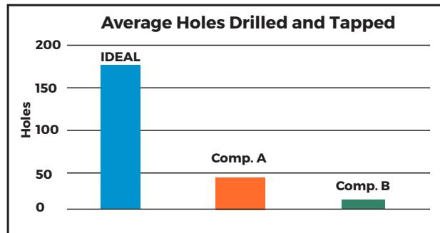
Based on testing 1/4-20 drill tap in 10 AWG Mild Steel
