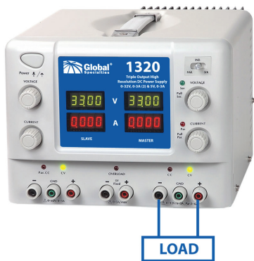
Figure 6. Parallel Tracking Mode
