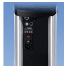
Model C RTC-C reference temperature calibrator with input for reference sensor and DLC sensor.
