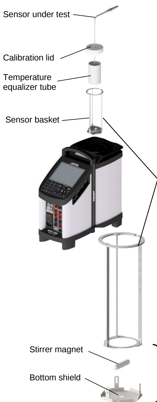
Fig. 2a Inserting the liquid bath kit RTC-168
