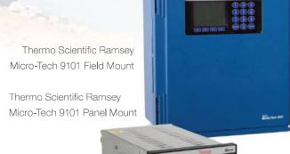
The Micro-Tech 9101 scale integrator electronics provides the intelligence to the weighing system, integrating output signals from the weighbridge and speed sensors to arrive at a rate of material flow and total material passed over the scale. The electronics also functions as the system power supply and incorporates all features that allow calibration, operation and diagnostics for the system.
