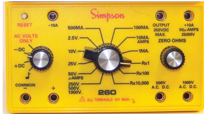
Figure 4-12. Jack and Switch Positions for Measuring Resistance
