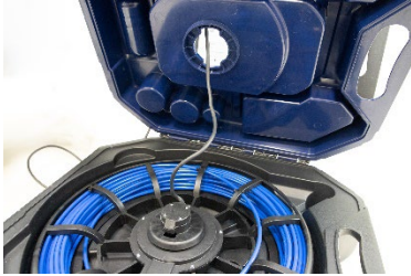
Fig. 60: Wrong: Camera cable not pulled tight
