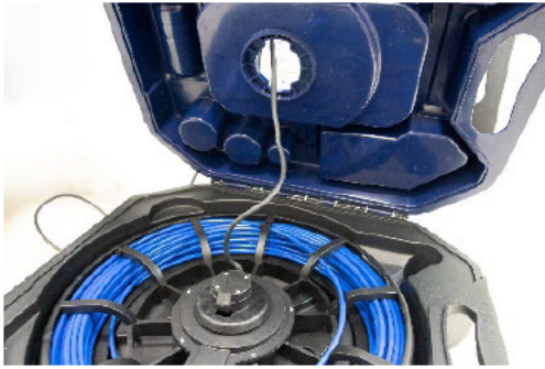
Fig. 60: Wrong: Camera cable not pulled tight
