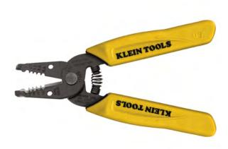
Complete electrical wiring tasks quicker by stripping 2 wires at a time with the Klein Tools 6-1/4-Inch Dual-Wire Stripper/Cutter. This tool is designed for use with 10-14 AWG solid wire. Its precision-ground stripping holes cleanly cut wire and aid in easy removal of insulation.
