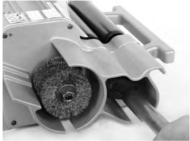
Figure 13 – Reaming I.D. of Tube
