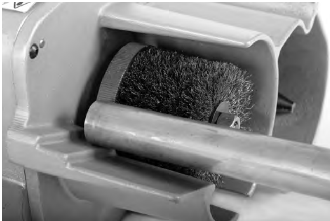
Figure 12 – Deburring O.D. Of Tube
