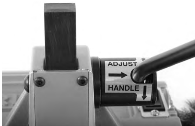
Figure 8 – Adjusting Handle Position
