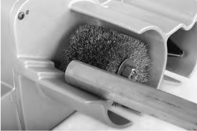
Figure 11 – Cleaning Tube O.D.
