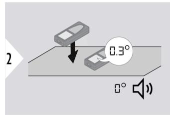
☞ Displays inclinations of 360°. Instrument beeps at 0°. Ideal for horizontal or vertical adjustments.
