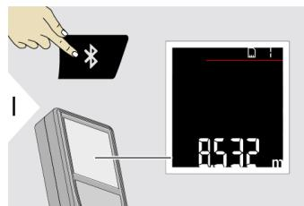
Press the Bluetooth key. The final measured value is sent to a connected device.
