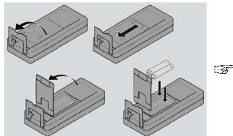
To ensure a reliable use, we recommend using high quality Alkaline batteries. Change batteries when battery symbol is flashing.
