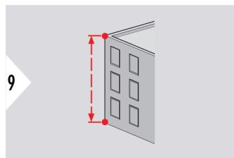
The result is shown in the main line and the measured distance above. Pressing the measuring key for 2 s in the function activates automatically Minimum or Maximum measurement.
