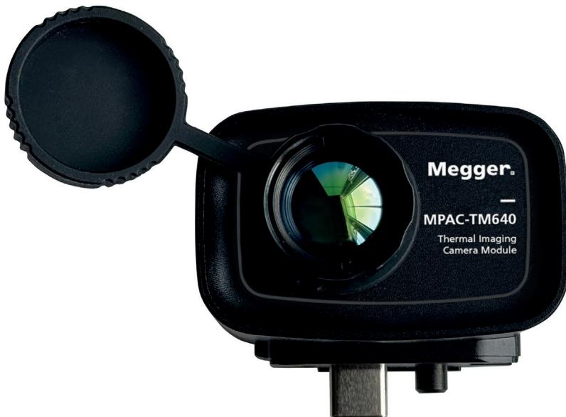
Plug in the thermal module at the top (refer image in 3.1) to be able to view thermal imaging screen on the display. If the thermal image is not clear, it is possible the focal length of the thermal module requires adjustment. The focal length of the thermal module is adjusted by turning the lens of the module.
