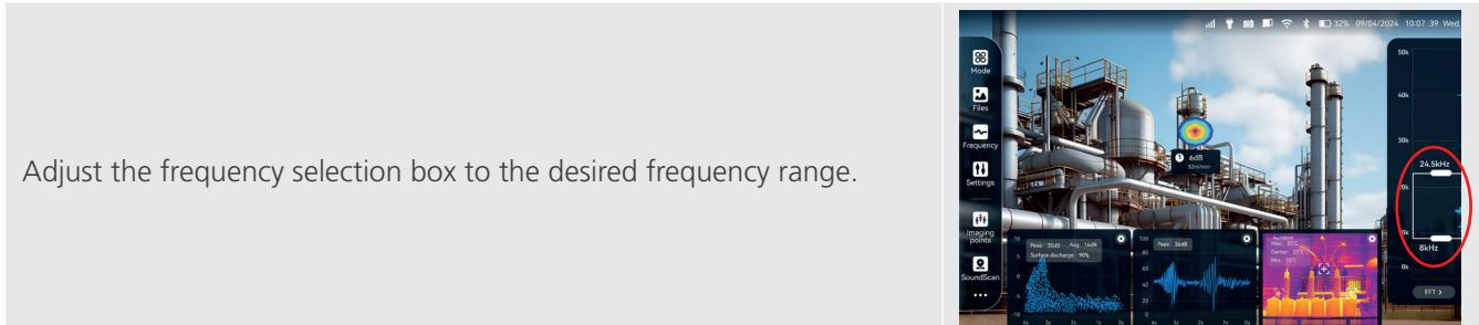
Adjust the frequency selection box to the desired frequency range.
