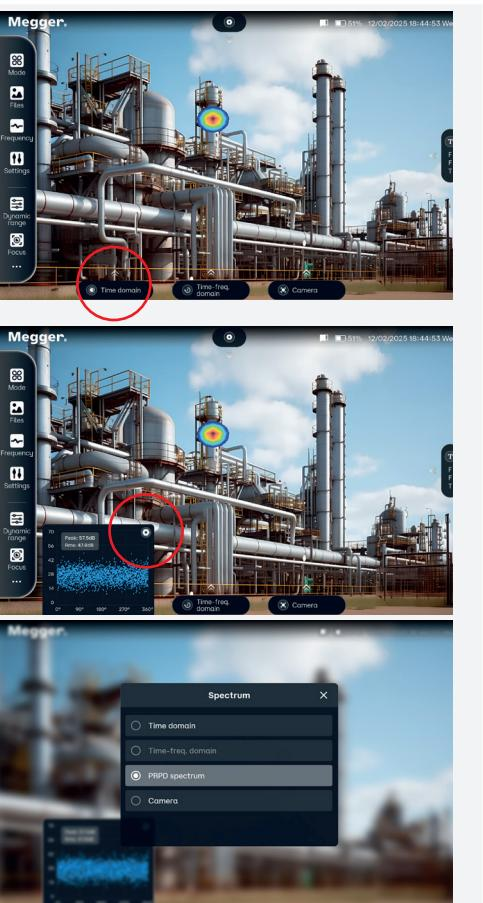
Three sub-displays are available on the MPAC cameras. Tap the tabs at the bottom of the screen to bring up the display. Tap the
