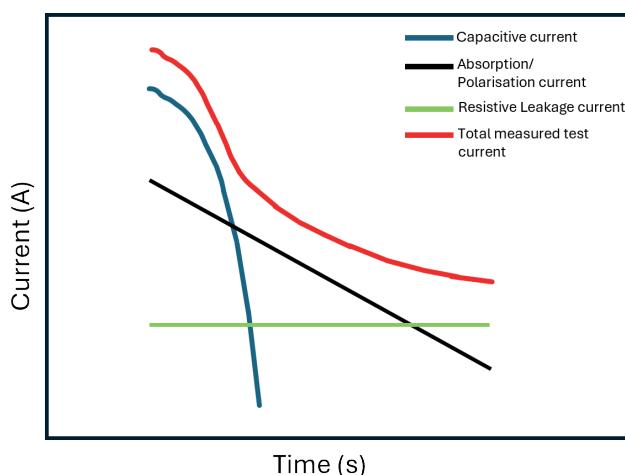
Separated curves for the three components of the polarisation curve
