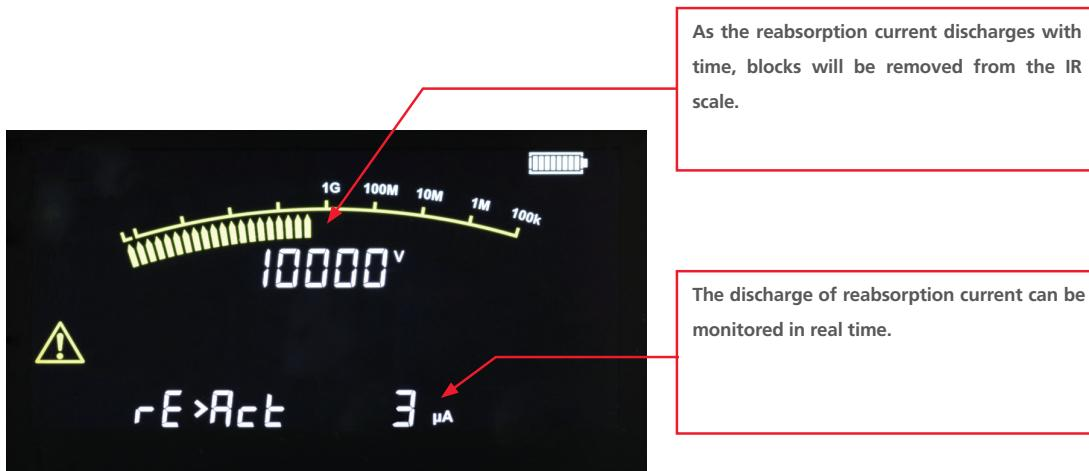
The accuracy of the IR measurement increases as the reabsorption current discharges. This is indicated by the reduction in the number of blocks on the analogue IR scale, as below:
