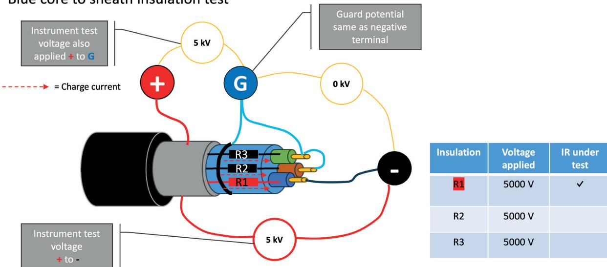
As can be seen, although the only insulation being tested directly is represented by R1 the test voltage is also being applied to R2 and R3, they are being charged, and an absorption current is flowing.
