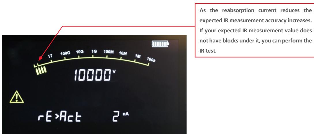
As a rule of thumb any part of the analogue scale which shows blocks means that IR measurements in this area will have a minimum of 10% additional error, but this can easily exceed 100%, as dictated by the physics of the still-present reabsorption current.
