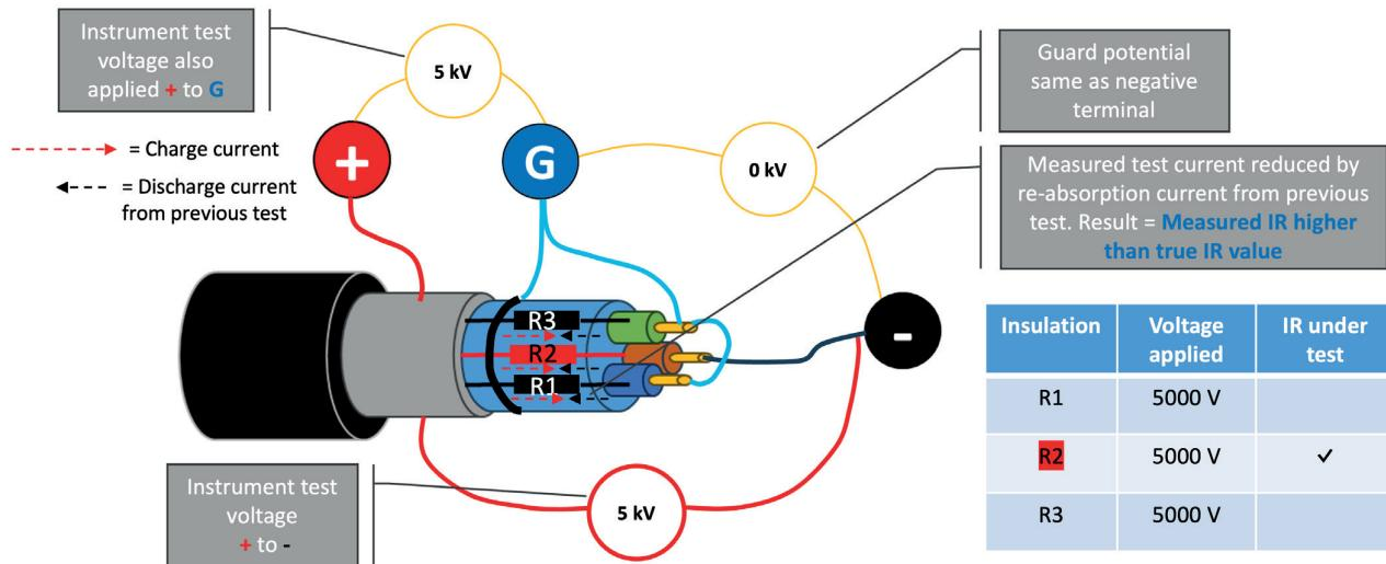
Again, care must also be taken that the reabsorption current is fully discharged to prevent a return voltage hazard. Please note that after a test the voltage measurement will only indicate that the capacitance has been discharged. Only the RE>Act™ test mode can monitor the reabsorption current.
