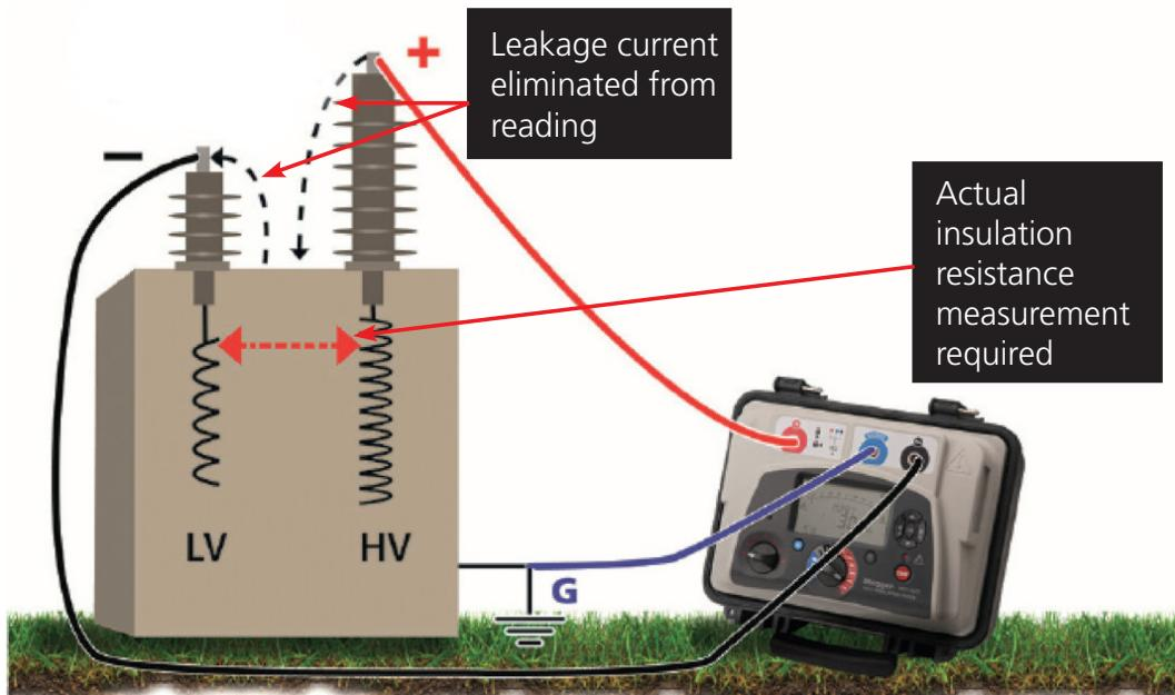
Above: a transformer winding insulation test, with the guard used to eliminate leakage current due to the surface path across dirty porcelain insulators.
