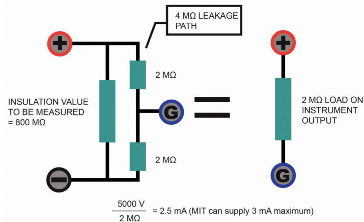
This circuit quickly demonstrates how an 800 MΩ insulation resistance can soon present a 2 MΩ load to the instrument with surface leakage. This is because the negative and guard terminals are at the same potential. High power of MIT range maintains the test voltage across the insulation and provides enough test current to accurately measure the insulation.
