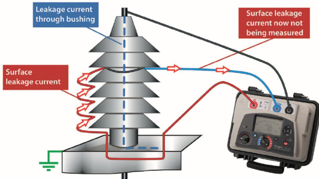
Wire has been wrapped around the centre of the bushing and connected to the guard terminal - now the surface leakage flows to the guard terminal. Current flowing into the guard terminal is not measured by the instrument and so is ignored by the insulation resistance measurement.
