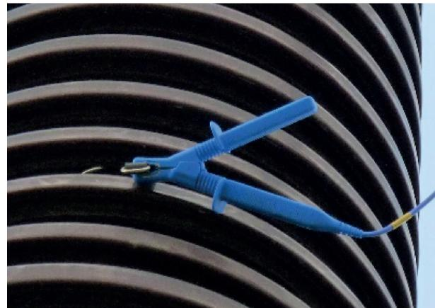
Here, an elastic conductive strap has been stretched around the bushing. The end of the straps has passed through the metal ring and secured with the lead clip.
