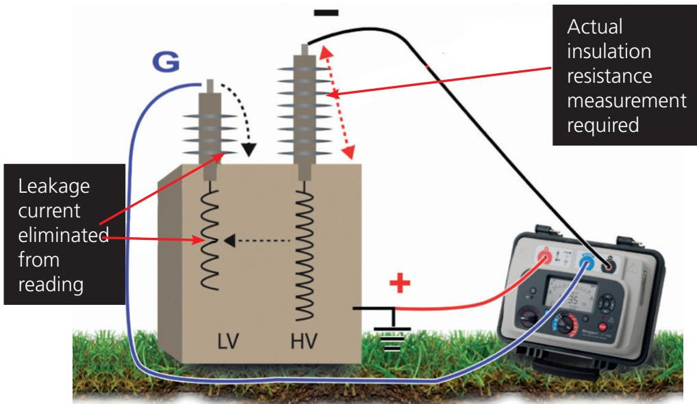
Above: the HV winding is measured without the effects of leakage current between HV and LV winding using the guard terminal.
