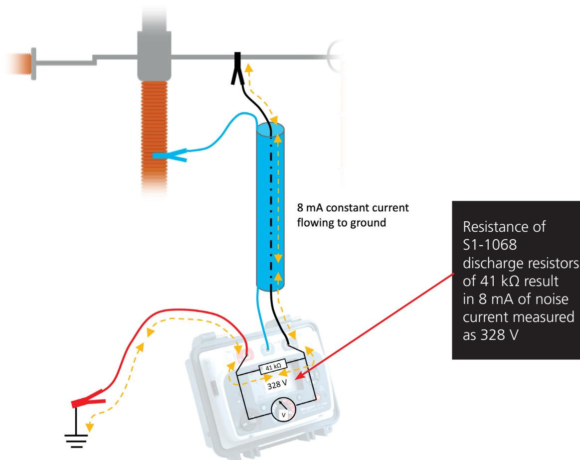
Once the test button is pressed and the IR test proceeds a relay is powered up to disconnect the discharge resistors (relay is powered open so it would fail safe in the event of power loss)
