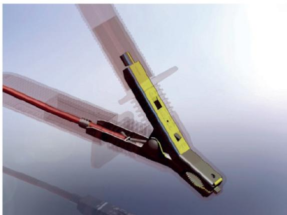
Even electrically isolated systems may exhibit significant capacitance, which will become dangerously charged by the application of the insulation test. Connections, including the leads and clips, should never be touched during the test. The system must be safely discharged before touching connections.
