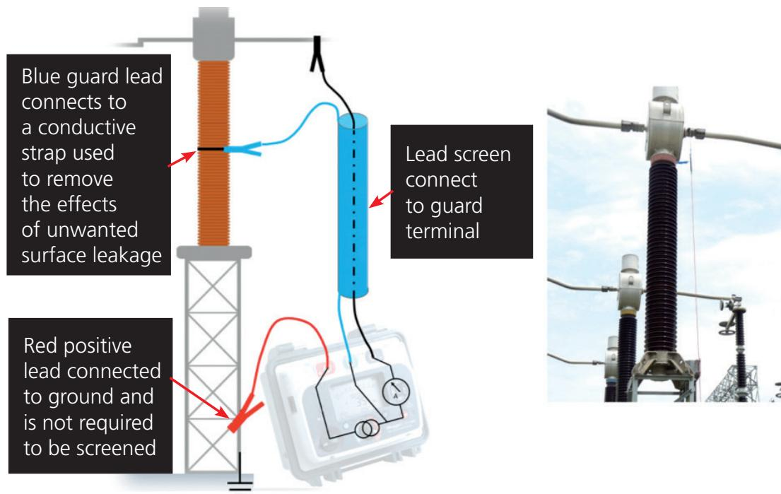
Some rules to observe when using screened leads in HV environments:
