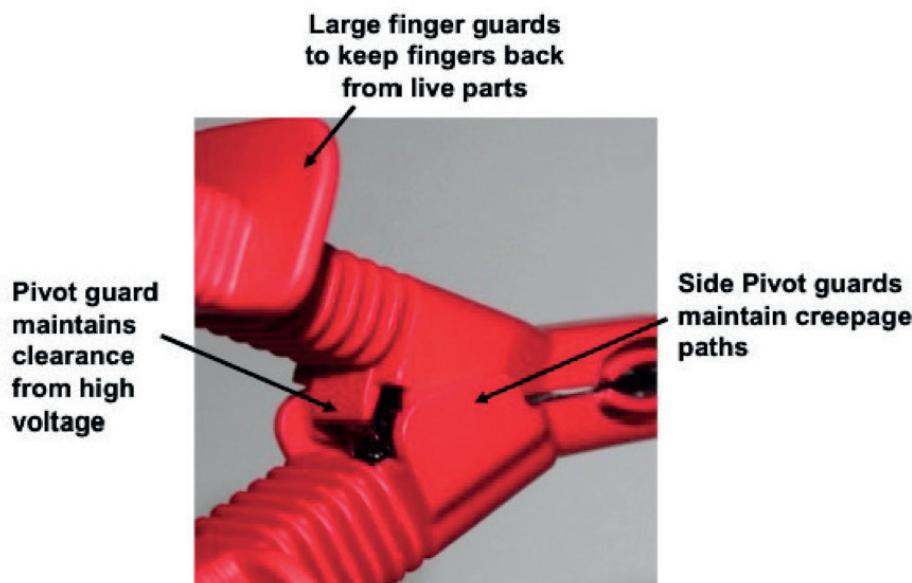
Test clip markings explained with respect to protection to instrument output:
