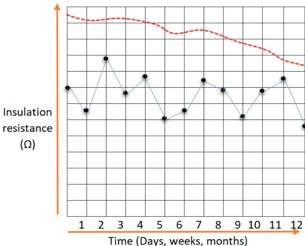
Sometimes the value of trending test results is not always apparent. However, this is usually because either temperature correction has not been performed, or it could be due to poor guarding of surface leakage or maybe inaccurate measurements from instruments unable to cope with noise or negative transient currents. However, by taking some steps outlined in this application note, results can be changed from those looking like the blue line, to those looking like the dotted red line.
