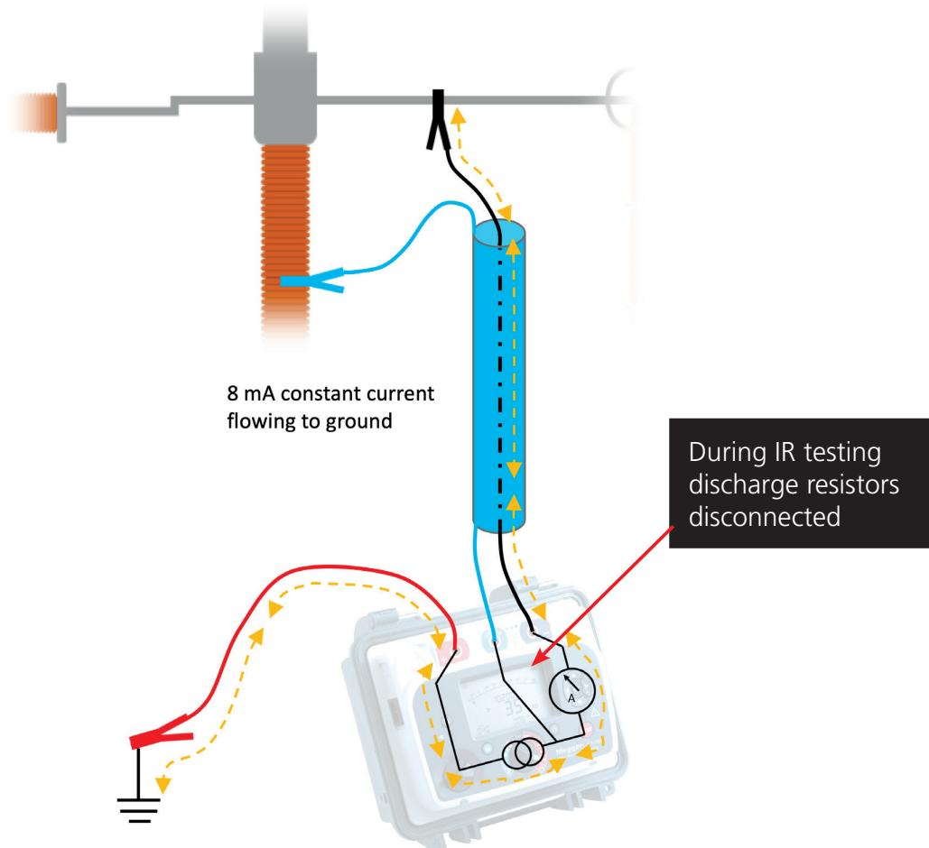
When the insulation tester is first connected the instrument will detect voltage and measure it as a safety warning. In this example an S1-1068 has a discharge resistance of  $41\text{ k}\Omega$ , so if 8 mA of noise current was flowing through the instrument to ground it would be measuring 328 V.
