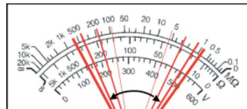
In high voltage environments such as 400 kV or 765 kV switch yards screened test leads are essential to obtaining good accurate measurements. However they cannot remove the effects of induced current on the test piece. In this case we rely on the instruments noise filters.
