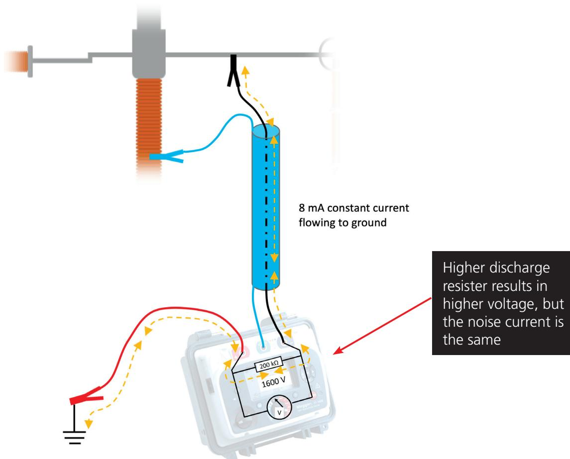
Some manufacturers use a much higher resistance in the discharge circuit to allow the use of lower power resistors. However as can be seen in this example it results in a much higher voltage measured.
