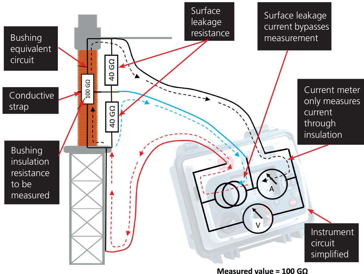
However the story doesn't end there. As you can see we have added example values to the above diagram. In this circumstance, any instrument within the Megger MIT or S1 range of insulation testers will provide measurements with no more than 1% additional error. This is an important part of the comprehensive specification these instruments provide.
