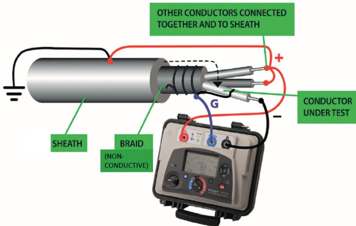
The guard terminal is connected to wire wrapped around the exposed insulation to pick up surface leakage. To measure insulation between one core and sheath only:
