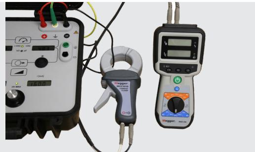
Connect the sync cable between the receiver and transmitter
