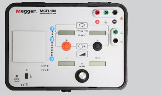
Connect the red terminal to the positive side of the battery string.
