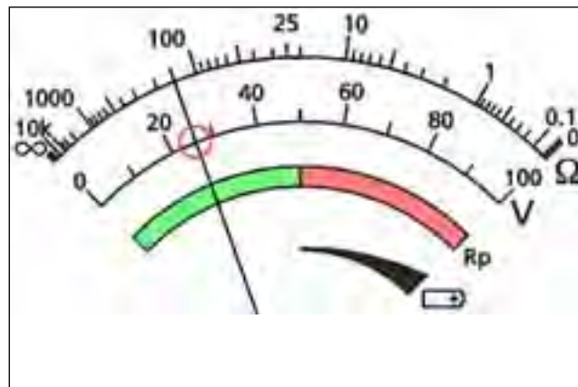
Figure 12: example ground noise voltage reading
