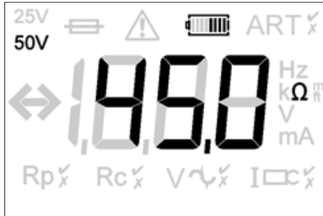
Figure 14: example two-terminal resistance reading (DET4 display shown)
