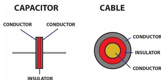
The longer the cable, the greater the surface area of the conductors and the higher the capacitance.
