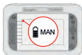
Current operational state. Currently in Manual operation
