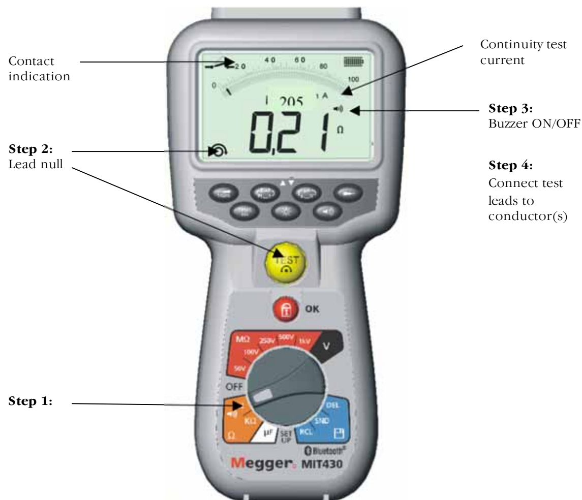
Figure 9 Continuity test and buzzer
