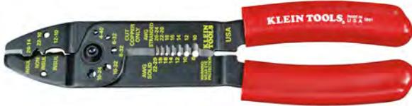
The Klein Tools Wire Stripper Multi-Tool cuts, crimps, and strips solid and stranded wire and shears bolts. Two cutting blades for 8-22 AWG solid and 10-26 AWG stranded wire. The crimping function handles 7-8 mm insulated and non-insulated terminals, lugs, and splices.
