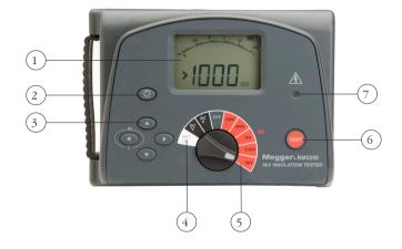
The BM5200 is turned on by rotating the main range switch to insulation test, voltage test or setup function.
