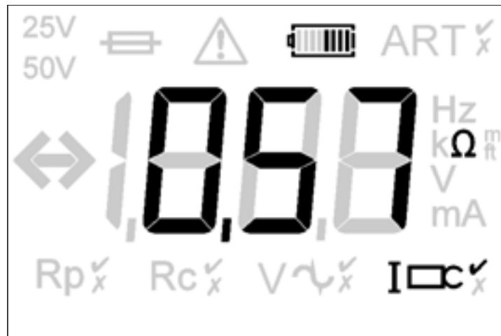
Figure 36: example resistance reading using two-clamp stakeless method
