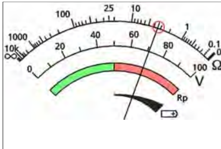
Figure 17: example two-terminal resistance reading
