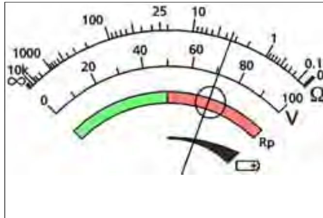
Figure 23: P stake resistance not OK (red region)
