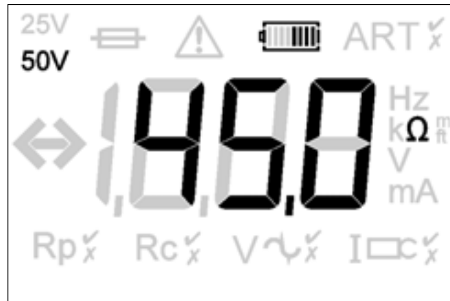
Figure 14: example two-terminal resistance reading (DET4 display shown)
