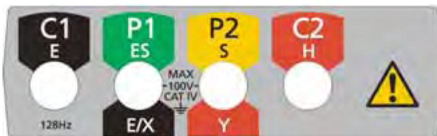
Test lead connections (at rear of instrument)
