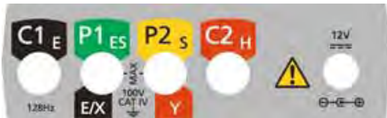
Test lead connections (at rear of instrument)
