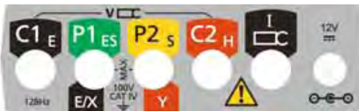
Test lead connections (at rear of instrument)
