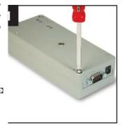
parate the two halves of e gauge housing by loosing the captive screws. ien pull the two halves art.
