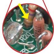
Twist the thermistor away from the resistor, or cut it out completely. Note the absence of the connection, identified by the yellow arrow. Then, install the new battery and reassemble the two halves of the housing.
