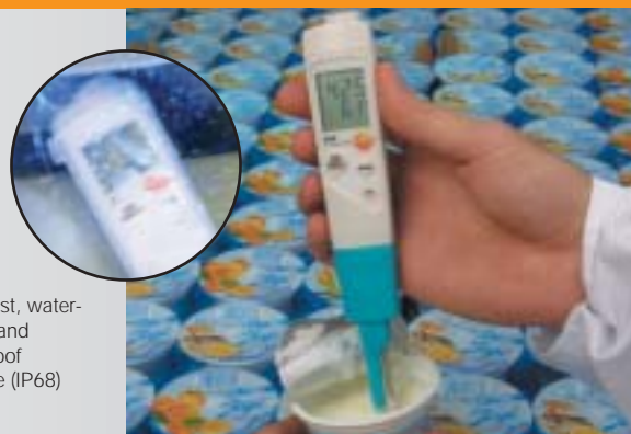
Spot pH check in intermediate storage facilities
