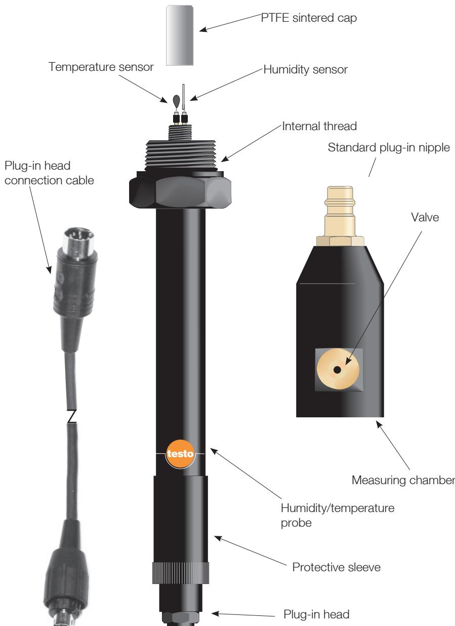
The two pressure dew point probes guarantee quick and accurate dew point measurement.
