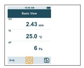
Depending on the connected probe, parameters can be configured for the measurement, for example, visibility of individual values or units.
