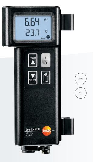
The testo 230 combines a complete pH measuring instrument and a full-value temperature measuring instrument in one compact splashproof housing. It reliably records pH values, reduction voltages and temperature in watery solutions as well as in semi-solid to solid media.
