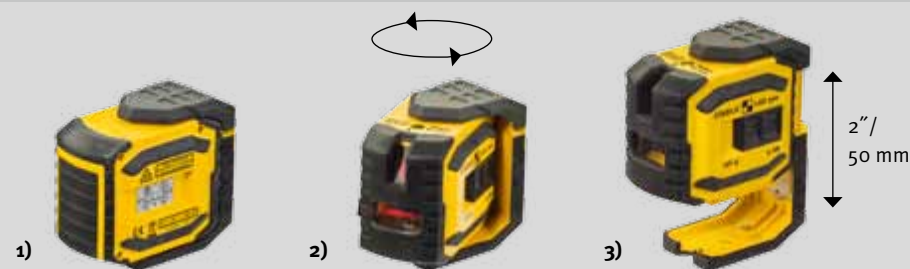
1) Park position. 2) The casing can pivot 360° inside the U-grip. 3) The extendable foot can be used to adjust the laser's height.
