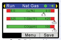
Tune-Rite ™ shows real-time data at steady-state so adjustments can be made to optimize appliance performance.
