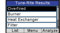
display a prioritized list of most likely potential issues to investigate. A drill-down into a "checklist" helps to keep track and record what has been inspected, adjusted, repaired or found to be an issue.
