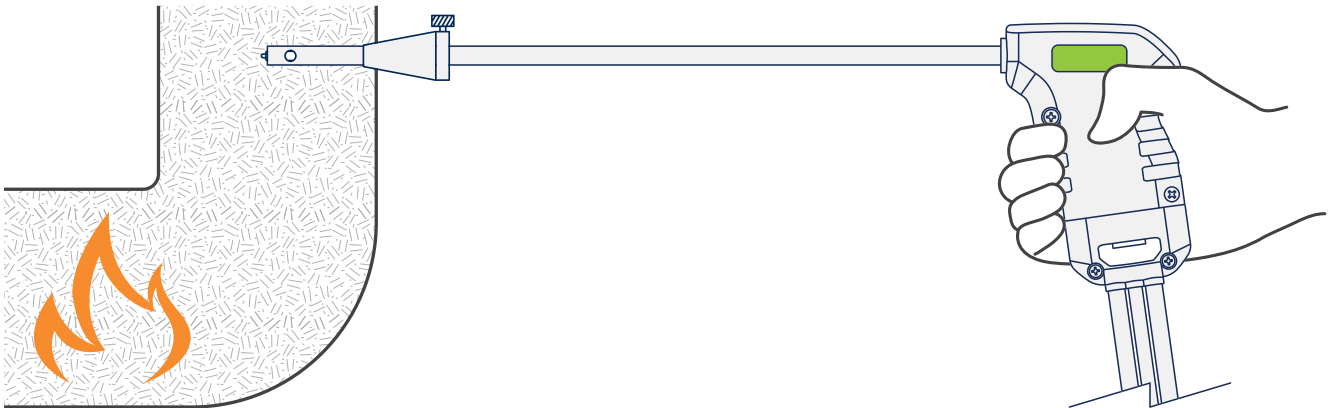
Fig. 3-6: Probe Placed in Center of Measurement Area
