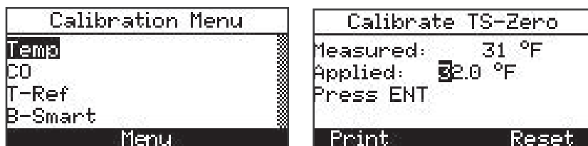
Figure 5-5: Calibration Menu & TS-Zero Calibration Screens
