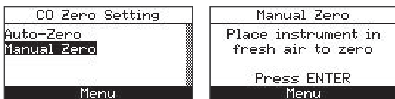
Figure 5-8: CO Zero Setting & Manual Zero Screens
