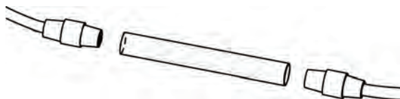
Figure 11. Removing End Plugs from Saturator Filter Tube
