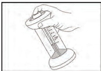
Figure 3. Venting FYRITE® to Atmosphere at 45° Angle
