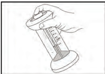
Figure 3. Venting FYRITE ® to Atmosphere at 45° Angle
